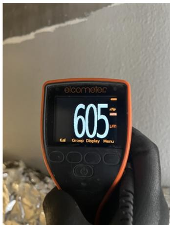
Completed application with coating thickness being checked.
