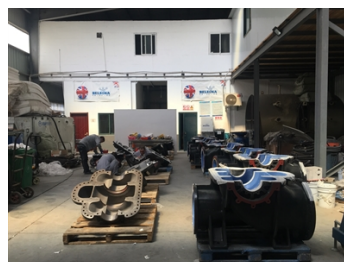
During application of Belzona 1341
