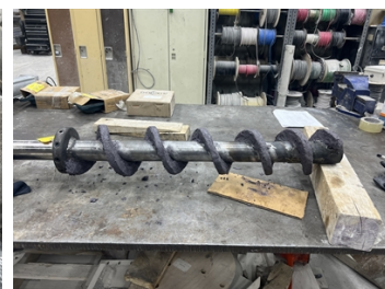
After application of Belzona 1812.
