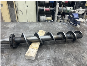
Screw conveyor before surface preparation.
