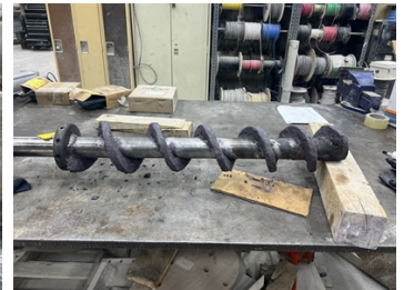
After application of Belzona 1812.
