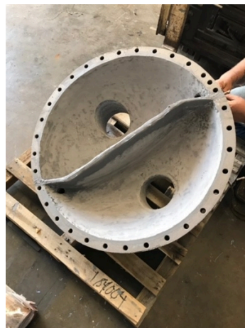
Rebuild Complete with Belzona 1111
