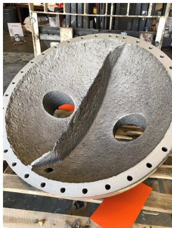
Completion of Abrasive Blasting
