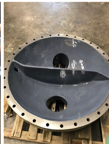
Complete Application with Belzona 1321
