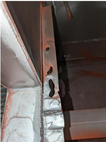
Vessel initially after chemical attack.
