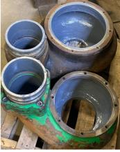
First pump with through wall after grit blasting.
