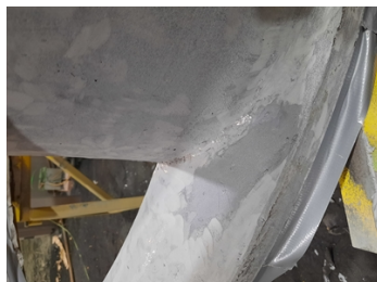
Resurfacing with Belzona 1111.
