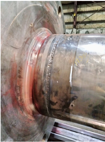
Shaft preparation completed for rebuilding
