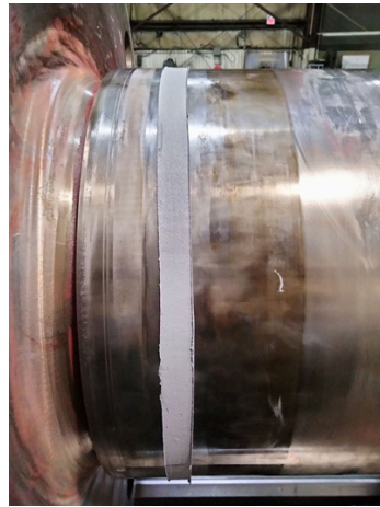
Belzona 1111 application finished and ready for machining
