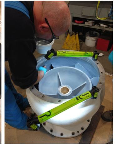
Preparation in progress for rebuilding of pumps bowls and suction bell as per the IFU
