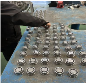
Metal former used to case nozzle inserts
