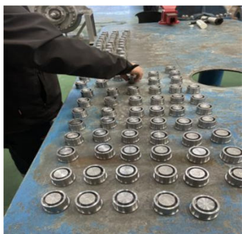
Metal former used to case nozzle inserts
