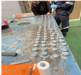
Application in progress of the nozzle inserts
