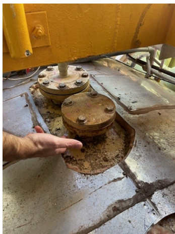
Severe through wall corrosion at the base of the nozzles exposed dangerous chemicals during the process
