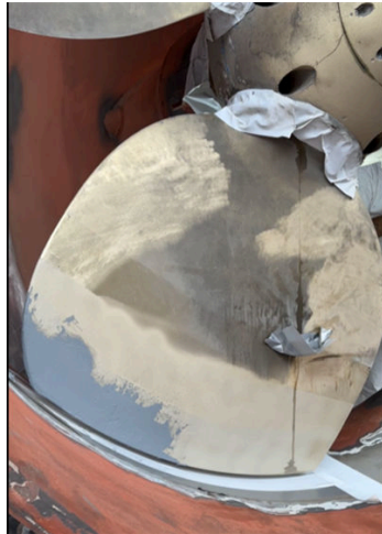
Belzona 1311 applied in areas of cavitation
