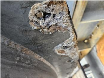
Flange with Sulfuric Acid Damage
