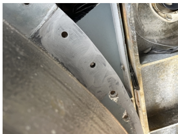
Flange After Repair with Belzona 4301
