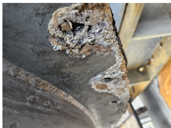
Flange with Sulfuric Acid Damage
