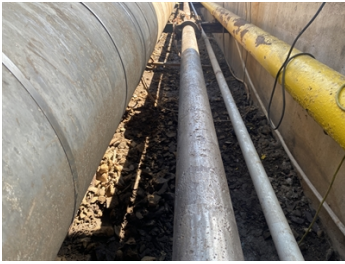
Corroded pipe used to carry ammonia.
