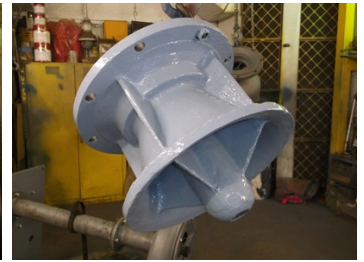
Protected with two coats of Belzona 1341N.
