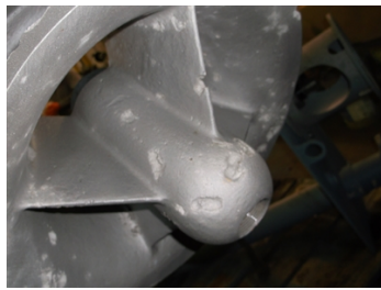
Grit blasted and ready for Belzona 1111.
