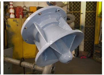
Protected with two coats of Belzona 1341N.
