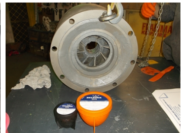
A look at the other side of the piece after the Belzona 1111 application.
