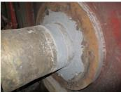
The gasket area former in place Application complete showing the initial clean up.
