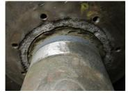
Showing the area of damage to The shaft former in place the shaft and gasket surface prepped.
