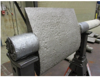
Pitting on the face.
