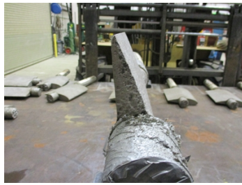
Pitting on the end.
