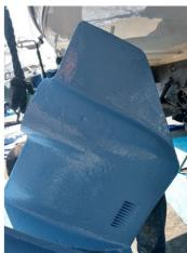
Belzona 1341 applied to protect the outdrives.
