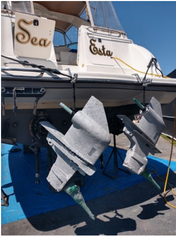
Both outdrives sandblasted and ready for application.
