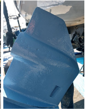
Belzona 1341 applied to protect the outdrives.
