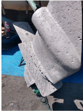
Up close, showing the erosion damage.
