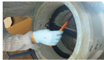
Applying Belzona 2111 to the gasket surface.
