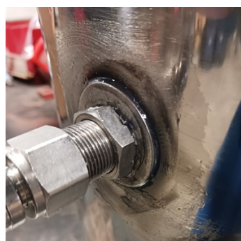
External fitting showing seal of Belzona 2311
