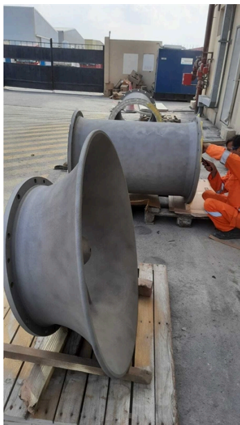
After surface preparation using grit blasting
