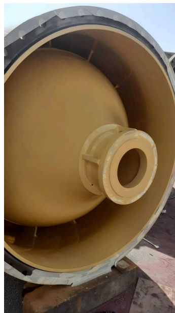
Application of first and second coat was completed and in this is the completed third coat application.
