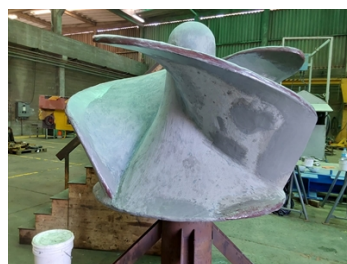
Application of Belzona 1121 (Super XL-Metal)
