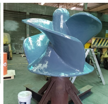
Coating with Belzona 1321 Ceramic S-Metal
