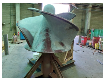
Application of Belzona 1811 (Ceramic Carbide)
