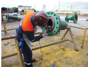
Surface preparation on the groove
