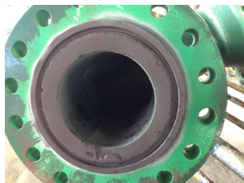
Damaged flange face due to high salt and H 2 S content
