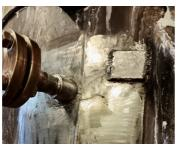
caused by a knock on the nozzle which created an impression and cracked horizontally. The crack was terminated by drilling a small hole at the end of the crack.
