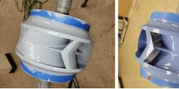
Impeller after the 1st coat with 2nd coat of Belzona 1341. Belzona 1341.
