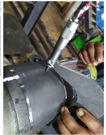
Smoothness, Tolerances checking (QA)
