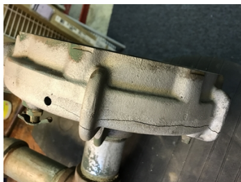
Depicts crack on pump casing.
