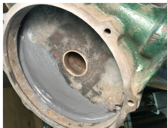
Inside of pump casing shows Belzona 1212 used to fill the crack and create a smooth finish for the water flow.
