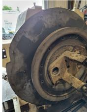
Mill face was grit blasted. Holes and pitting were filled with Belzona 1311
