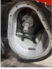
The final drive housing seat is not damaged, but it is out of alignment due to frame distortion. The mating surface former to create a new, will be cleaned and prepped with a mechanical blaster and all bolt holes corked, then Belzona 1111 will be applied over it.
