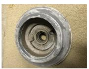
Belzona 1111 and Belzona 1212 The completed pump casing were used to build up corroded was successfully rebuilt with and eroded surfaces.
