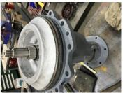
Belzona 1111 and Belzona 1212 then sanded by hand to create a consistent annular surface suitable for reassembly with the impeller and the mating casing.
