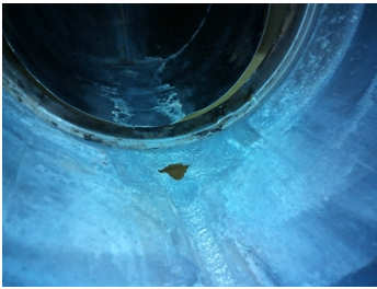
Damaged bottom and walls of the boiler.
