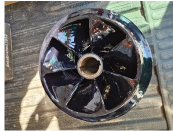
Application of Belzona 2141 (ACR-Fluid Elastomer)
