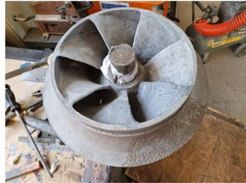
Filling damaged blades with Belzona 1311 (Ceramic R-Metal).
