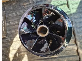
Application of Belzona 2141 (ACR-Fluid Elastomer)
