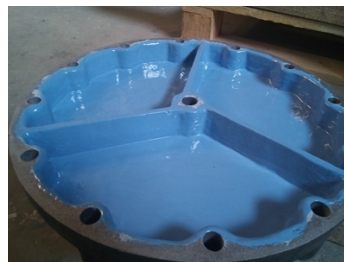
Repaired and protected cover.
