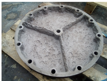
Heavily damaged exchanger cover
