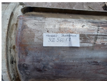
Damaged shaft under the bearing.
