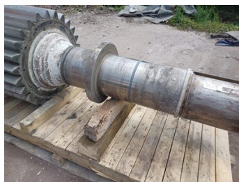
Shaft after repair
