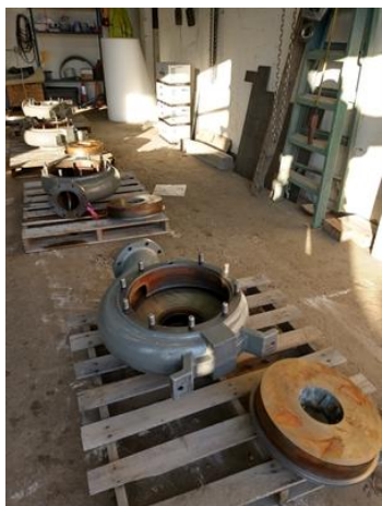
Brand new pumps ready to be coated.
