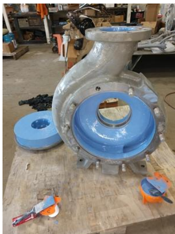
First coat of Belzona 1341 applied.
