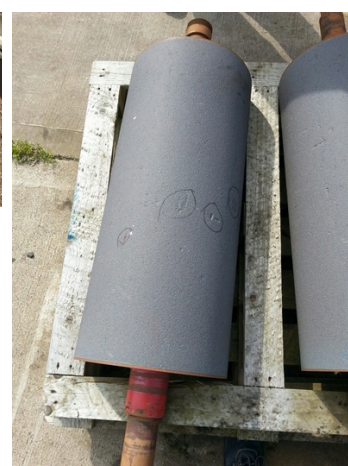
Roll crushers machined & put into service. Image taken 18 months, minor damage noted.
