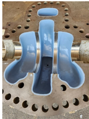
Pump casing protected with Belzona pump coating
