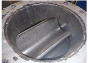
The rotor whilst still in it's original housing
