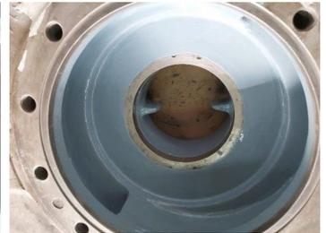
Once the surface was rebuilt, Belzona 1321 (Ceramic S-Metal) was applied to enhance protection and prevent further damage.
