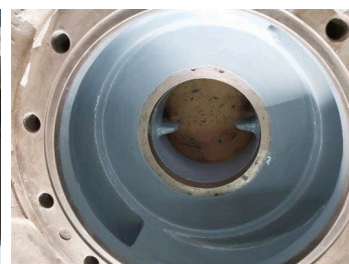
Once the surface was rebuilt, Belzona 1321 (Ceramic S-Metal) was applied to enhance protection and prevent further damage.
