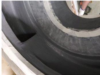
Surface preparation on the pump before the application of Belzona system
