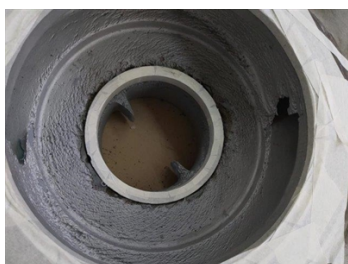
Erosion evidence on pump component due to high solid content
