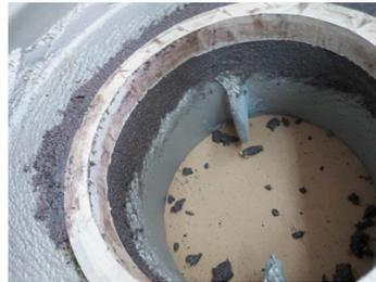
Pump surface was rebuilt with Belzona 1311 (Ceramic R-Metal)
