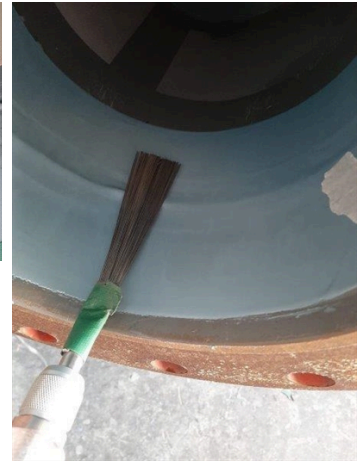
Spark testing in progress to detect pinholes for a flawless protective coating.
