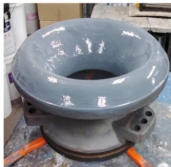
First coat of Belzona 1321 applied.
