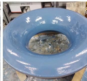
Pump housing complete with final coat of Belzona 1321.
