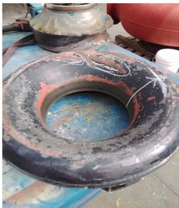
Damaged pump housing.
