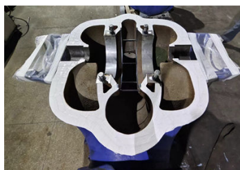
Protection of matching surface before surface preparation
