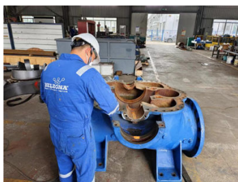
Degreasing and chamfering pump casing surface
