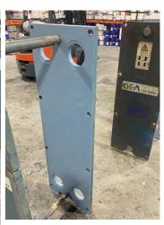
Areas to be rebuilt/coated were checked for chlorides, chlorides were neutralized to acceptable levels, units were blasted and profile checked as per product manufactures recommendations.
