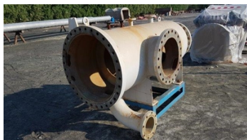
Sea water strainer suffered corrosion on the internal surface
