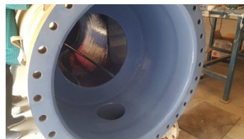
The internal surface of the strainer was rebuilt with Belzona 1111 (Super Metal) and overcoated with Belzona 1341 (Supermetalgilde)
