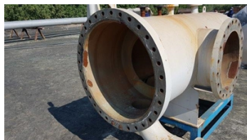
A closer look at the corroded sea water strainer
