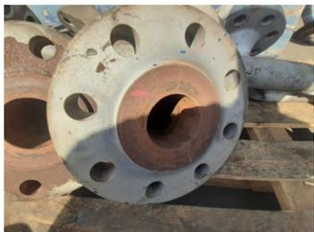
Worn-out flange face need repair
