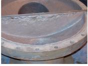
The attached image showcases Bar stock serves as a precise a severely eroded division bar on a heat exchanger end cover. (Ceramic R-Metal) is expertly This type of damage compromises the component's the damaged area to its performance and efficiency, highlighting the critical need for effective and durable repair solutions.
