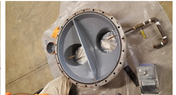
Protection completed with Belzona 1321.
