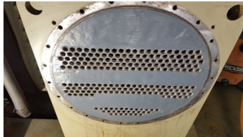
Rebuilding and protection completed with Belzona 1121 and Belzona 1321.
