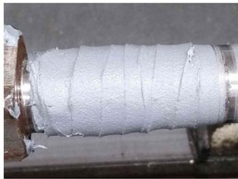
Application of Belzona 1111
