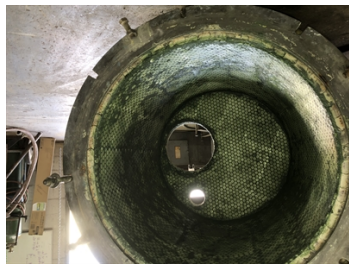
Grout completed with Belzona 1813.
